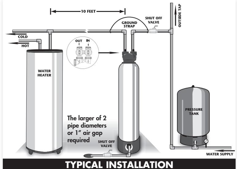
2. The tank should be installed on a firm, flat surface (above or below grade).
